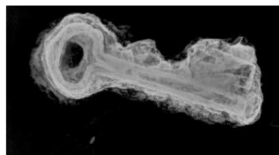
Iron key revealed inside lump of rust by x-ray.
